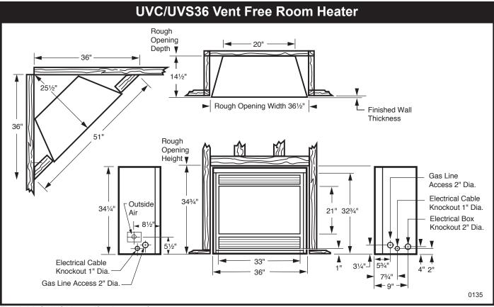
Fig. 1 UVC/UVS36 specifications and framing.
